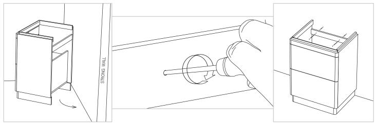
It is recommended that the unit and basin are secured to a suitably reinforced wall to ensure stability. This should be done using the wall hanging plates supplied. The wall fixings supplied are intended to be used on a solid brick walls. Check suitability before continuing.
