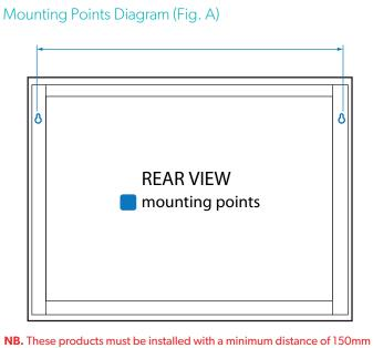
between the infra-red sensor switch and any adjacent wall or object to ensure correct operation of the sensor.
