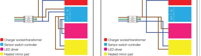
Rewire the mirror as shown in the diagram above. HiB recommends that all electrical bathroom products should only be fitted by a suitably qualified, Part P registered electrician.
